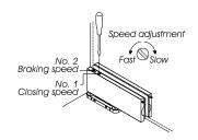
Introducing the **MORITZ** self-closing patch fitting for internal frameless glass doors. Compact and slim, it represents the latest refinement in floor-mounted closing for doors.
